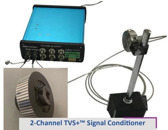
2-Channel TVS+™ Signal Conditioner with TVS+™ optical probe (main) and shaft coupling with TVS+™ label (insert)
