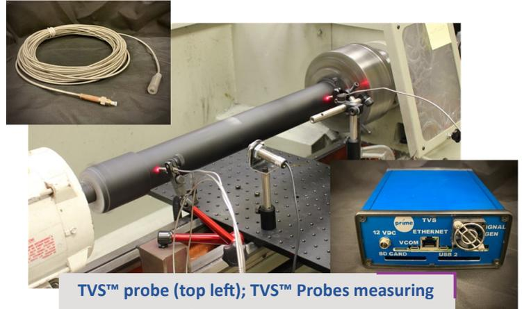
TVS™ probe (top left); TVS™ Probes measuring a shaft (center); 2-Channel TVS™ Signal Conditioner (bottom right).
