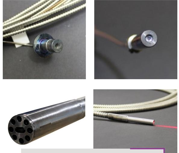
Clockwise from top left: Right Angle Probe; Front Window; Standard Lensed Probe; Gas Cooled Probe
